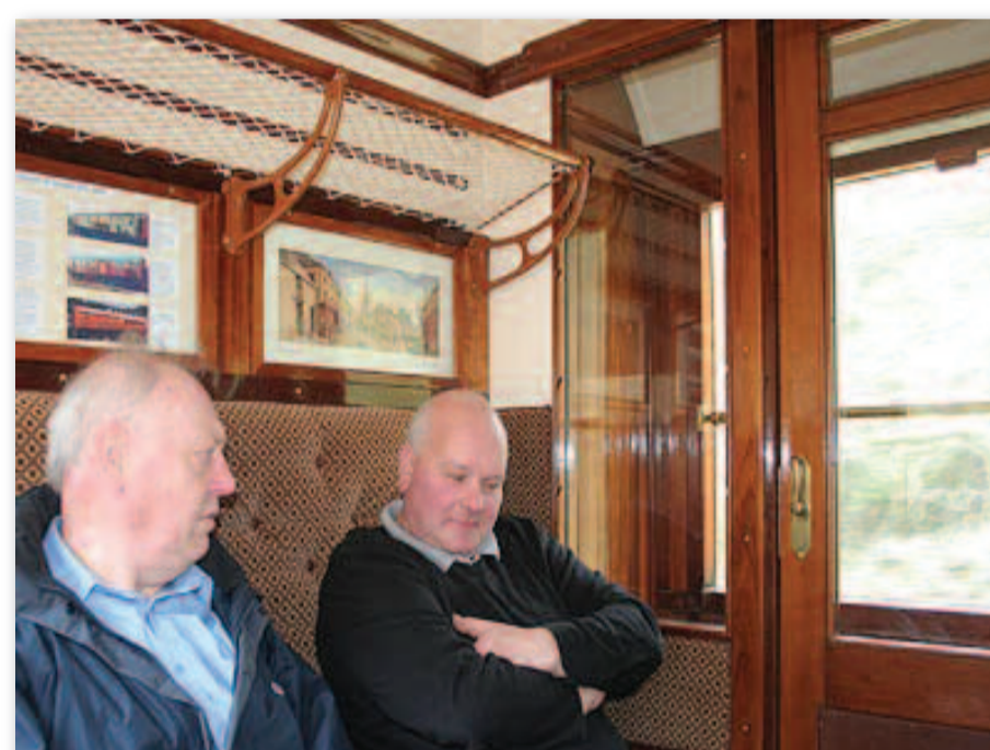
Attention to detail in the interior, both in the guard's van section and in the compartments, is commendable. The seating moquette was specially made to the original specification, as were all the fittings. On the right is co-owner Marcus Woodcock in conversation with Dave Simpson from the Scottish Railway Preservation Society who painted Thompson Third Corridor 1623 in scumble (teak).
