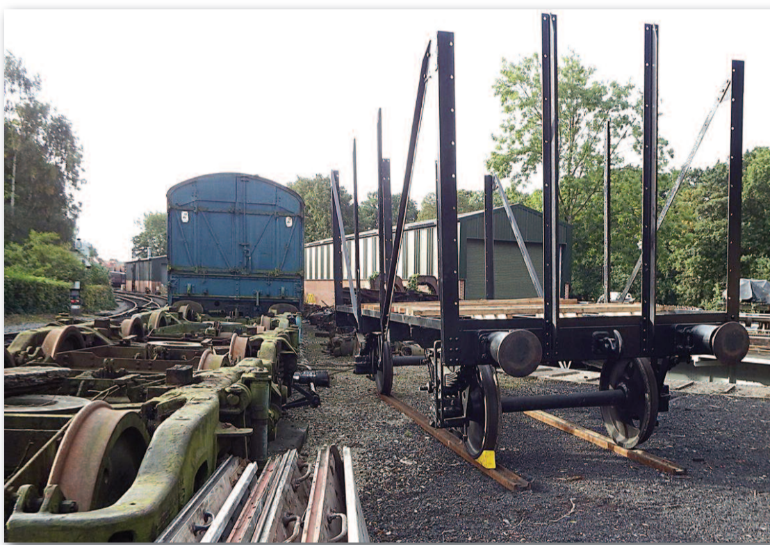
Bit of a job on here! Like all LNERCA projects, we inevitably go back to basics as shown here. The underframe sits on its isolated track awaiting the rebuilding of the bodywork.
