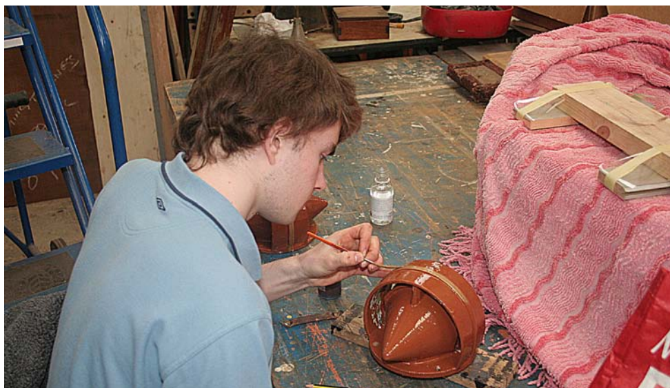
With his long-haired brush - and steady hand - Christopher Johnson puts the gold lining on the top of a ventilator which will be fitted on the roof of East Coast Joint Stock No. 189. Photo: Murray Brown.
