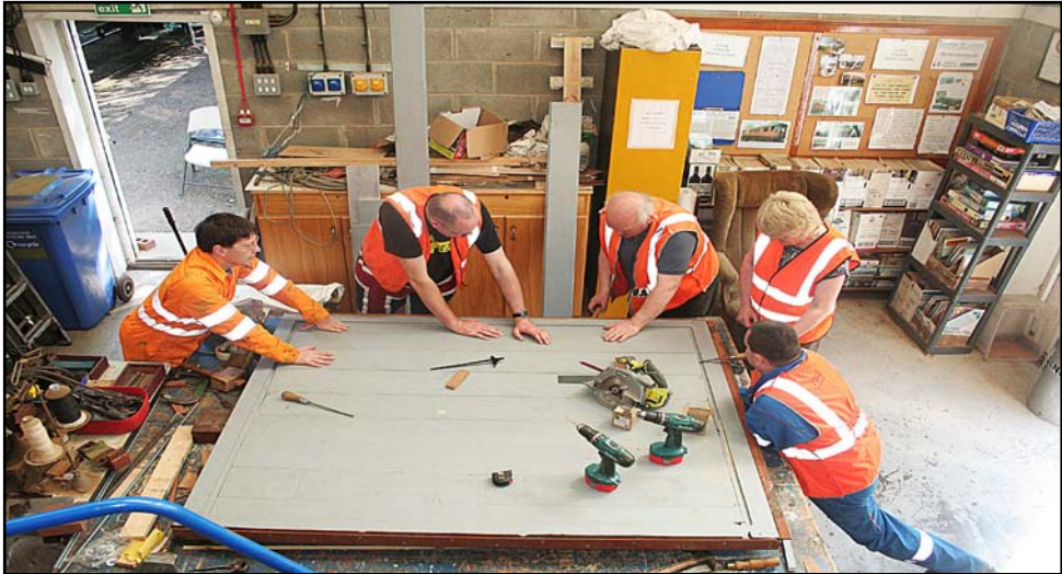
One of the brand new doors for the Covered Carriage Truck, nears completion inside the Atkins shed as the last tongue & groove board is slotted into place.
