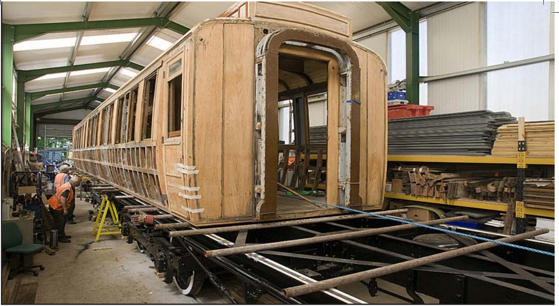
The body of 189 begins its journey, courtesy of numerous boiler tubes ex Q6 63395, a ratchet, a nylon rope, ten worried volunteers and a strict Foreman, Marcus Woodcock! Photo: Gary Lyne.
