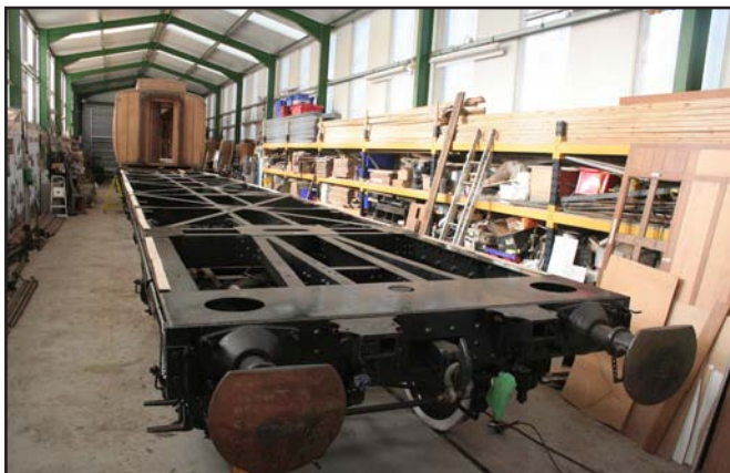
Its taken 17 years for the 'Perth' underframe to come in useful. Built in 1926 for BTK 62540, it ended its BR days as a Departmental vehicle (ADE 320692 & Internal User 096060) at Perth. The SRPS had the body and we had the underframe. It awaits the body of 189 being rolled onto it.
