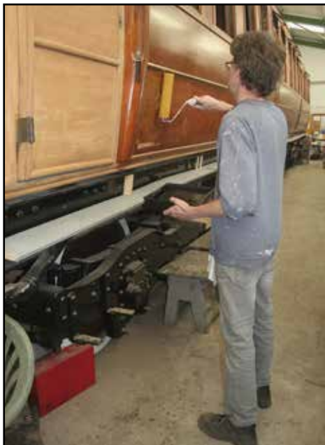
The first coat of varnish is applied on September 30 - Russ Whitwam wields the roller. The varnish is then brushed.
