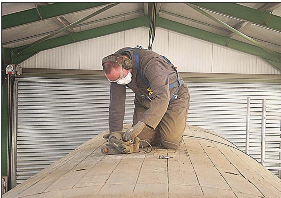
The Atkins shed is full of masked men! Bedecked in safety gear, Gary Lyne undertakes one of the less pleasant jobs - that of sanding the CCT's roof to remove old debris and also to ensure the new roof sheet is not pierced by intrusions which would allow water ingress. Photo: Murray Brown.
