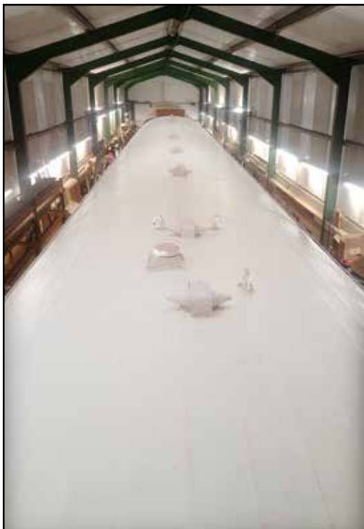
Several coats of Sikaguard have transformed 43567's roof. What a shame we couple steam locos to it! Photo: Gary Lyne.
