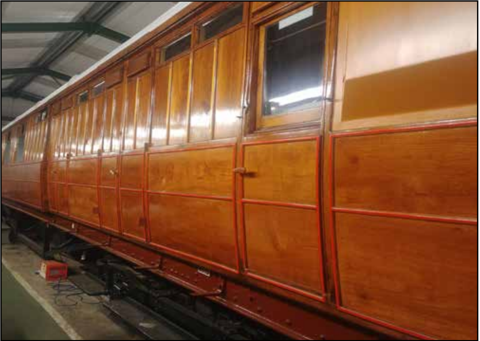
It's looking good but nowhere near finished. Still to have at least five more coats of varnish and the primrose lining added, 43567 nevertheless is looking far better than when it entered the Atkins shed. Photo: Gary Lyne.
