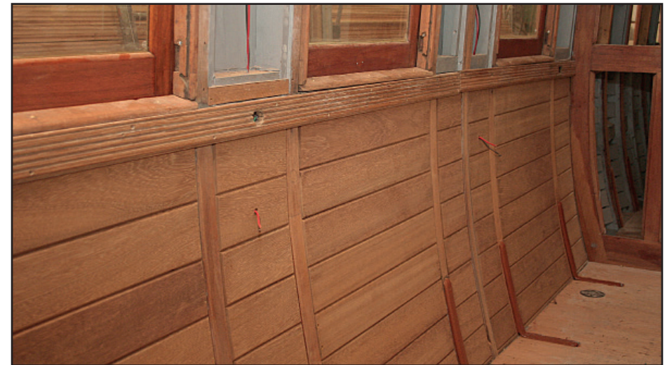
Looking good: With matchboarding now in place and soon to be varnished, the interior of 189 is looking like it did when we first took delivery - except underneath is so much better. Photo: Murray Brown.
