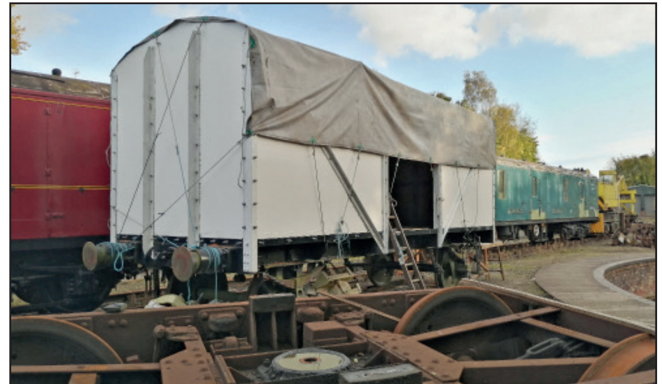
By October 7, the ends were in place, as were most of the carlines, so allowing a tarpaulin to be placed over the vehicle. This then allowed work to continue in inclement weather. Photo: Andrew Daniel.
