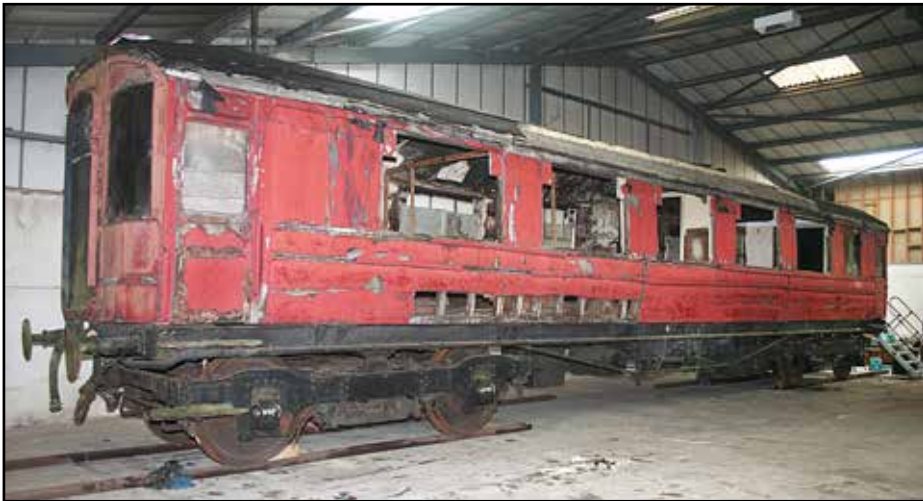
First carriage installed was NER First Open 2118 on May 3 which had come the 13 miles from a farm at Barton Hill where it had resided for seven years. The moving of 2118 into the industrial premises means the carriage is under cover for the first time in over 40 years. It is in extremely poor condition and an assessment is to be made to see what can be done to conserve it, pending a rebuild. Photo: Murray Brown.
