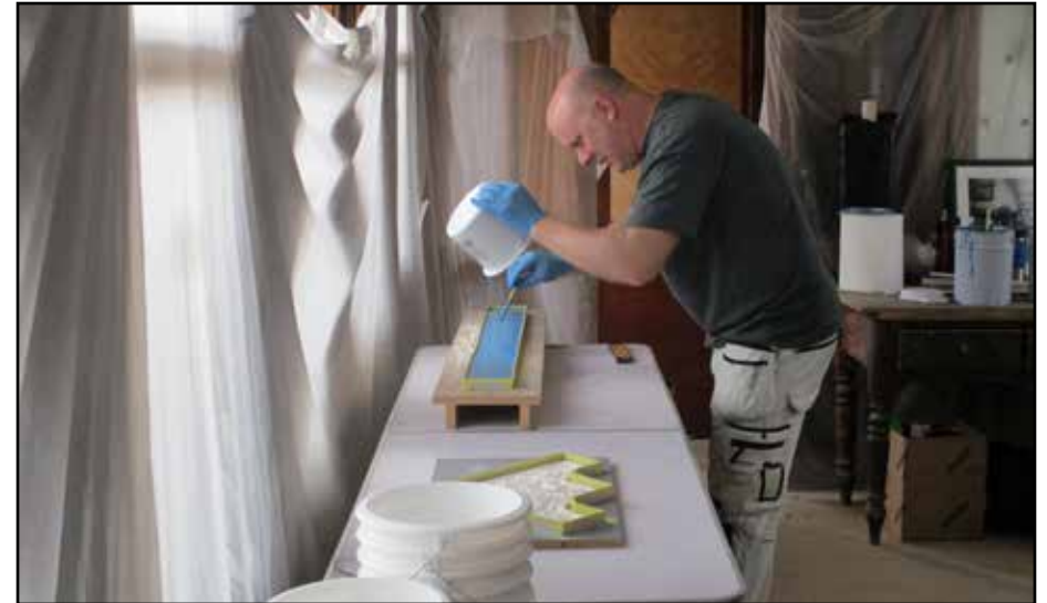
Frank Holmes makes a mould in connection with the manufacture and fitting of the Lincrusta friezes in 189. The next Newsletter will contain a feature on this remarkable process. Photo: Phil Brunson.
