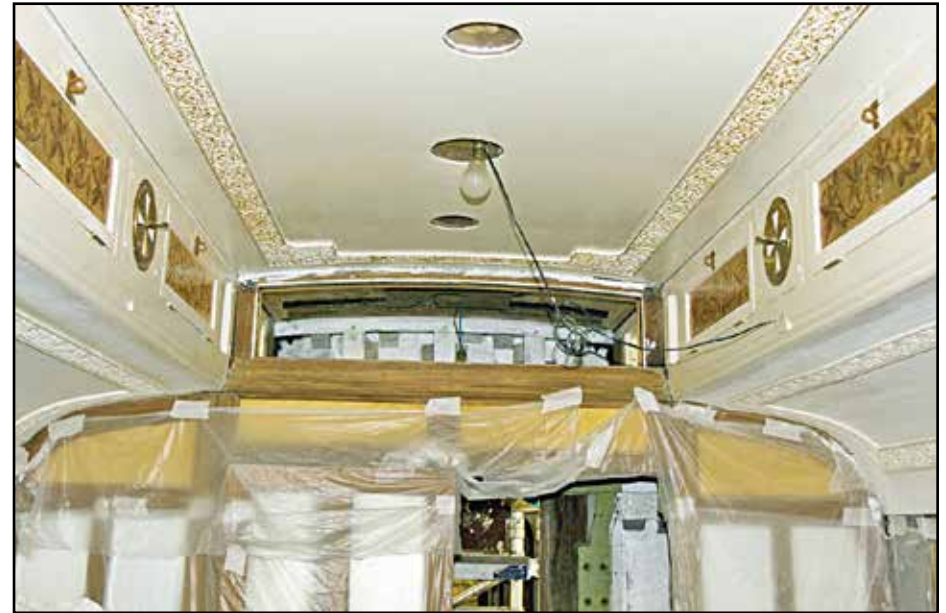
By the end of 2021, the lincrusta on the main saloon upper ceiling had received gold leaf in all its splendour, giving an indication how magnificent this carriage will look when finished.
