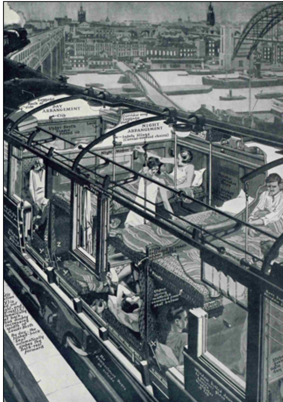
This cut-away diagram which appeared in 'The Sphere' clearly shows how a top bunk folded down to allow two passengers to lie down, one above the other. Of interest the train is crossing the High Level Bridge, Newcastle.
