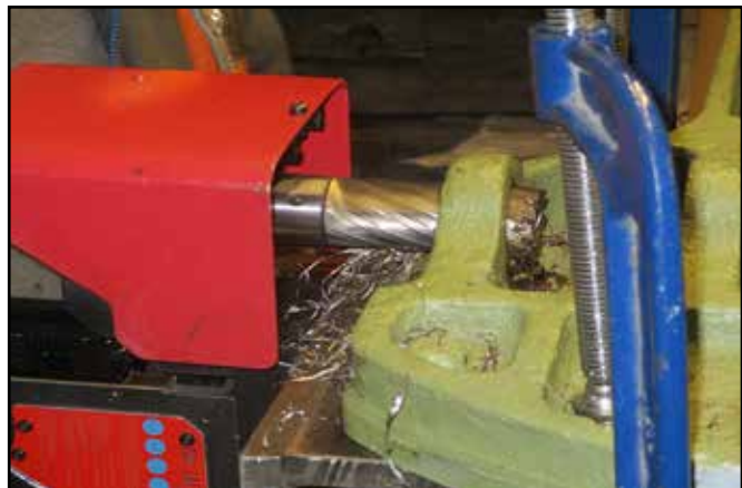
The green gangway end is pictured having one of its lower fixing pin holes bored to enable a new bush to be pressed in. Photo: Phil Brunsden.
