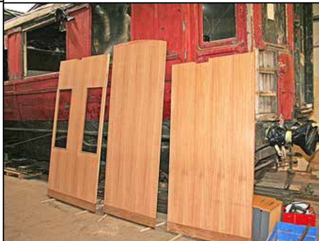
New panels are being fabricated where needed for TK 23896. On the left is part of the corridor screen, centre is a compartment partition and right, a toilet wall. Photo: Murray Brown.
