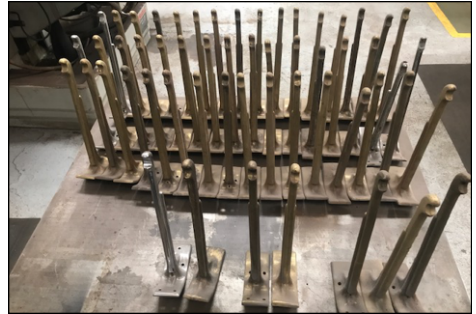
These are some of the brass luggage rack castings being prepared for chroming. Sufficient are to be ordered to enable three of our carriages to be fitted. Photo: Nick Stringer.
