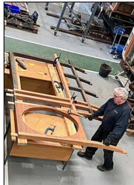
Left: In the Kirby Misperton Unit 10 workshop, Jim Chittock puts the finishing touches to the new framing, the centre piece being the Thompson trademark – the oval window, such a distinctive feature of this designer's carriages, for the Composite Lavatory (CL) 88339.
