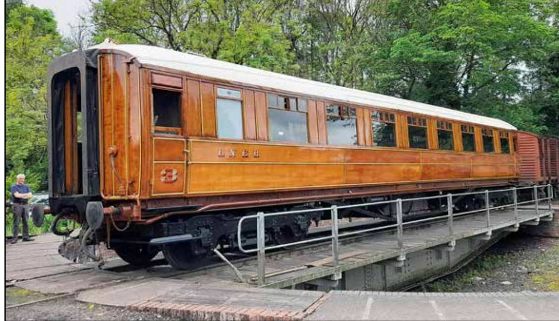
Looking magnificent, inside and out – TTO 23956 is pictured on the turntable after exiting the Atkins shed on May 23. Admiring the carriage is the gentleman credited with undertaking a large amount of the varnishing and intricate lining-out of the half-round mouldings along both bodysides – Ian Hollis. Photo: Marcus Woodcock.
