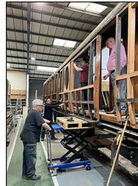
Left: In the Kirby Misperton Unit 10 workshop, Jim Chittock puts the finishing touches to the new framing, the centre piece being the Thompson trademark – the oval window, such a distinctive feature of this designer's carriages, for the Composite Lavatory (CL) 88339.
