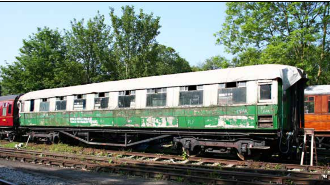
Pictured in Pickering yard on June 10, 2006, the carriage had to wait well some 15 years since arrival in 2002 before thoughts turned to converting it for wheelchair users. As arrived, the external panelling was a mixture of plywood and teak as the annotation shows. The somewhat unprofessional white lettering was later obliterated and replaced by a sign in a window, orchestrated by the LNERCA's former signwriter, Len Clarke. Photo: Murray Brown.
